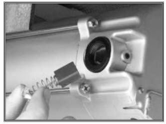
Figure 55. Carbon brush and spring.
